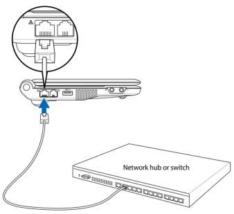
Network cable with RJ-45 connectors
